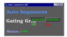
2. Click on the "Grid On" button. This will run a program to set all the GG power supplies. You should see the message "Downloading Setpoints". It should take ~3 minutes for all sectors to come up to voltage. When the gated grid is ready, all sectors on the main screen turn green:
