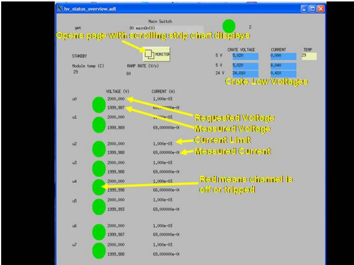
Figure 4. Illustration HV Status Overview GUI.
